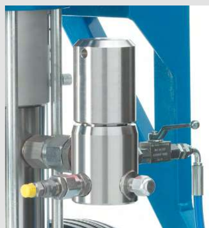
Standard high pressure filter on the pump outlet
